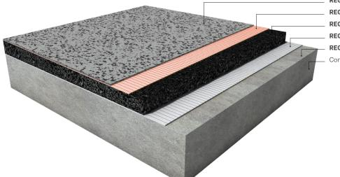
REGUPOL everroll rubber floor REGUPOL adhesive 41-103 (red) REGUPOL sonusfit m513 underlay REGUPOL adhesive 43-102 (blue) REGUPOL primer 90-102 (white) Concrete slab prepared to AS1884
